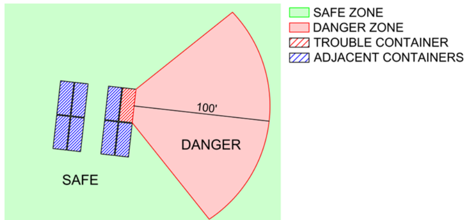
Figure 24 Exclusion Zone Exterior Container
