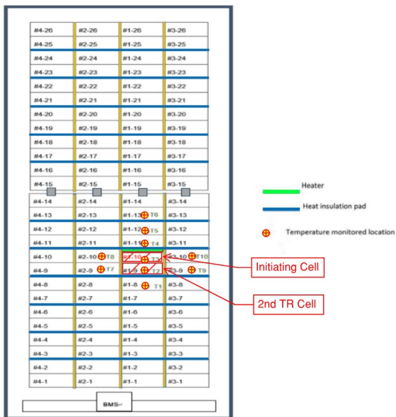
Figure 8. Module Level Test Thermocouple and Heater Positions
