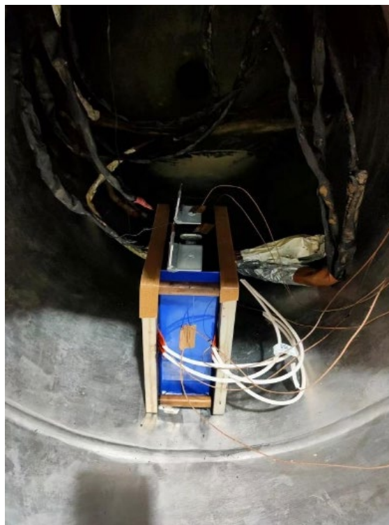
Figure 7. Battery Gas Composition Test Chamber
